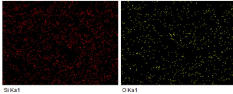
Figure 5: EDX and mapping of the EDX of Pasir Tumboh of 950 °C at x50 magnification
