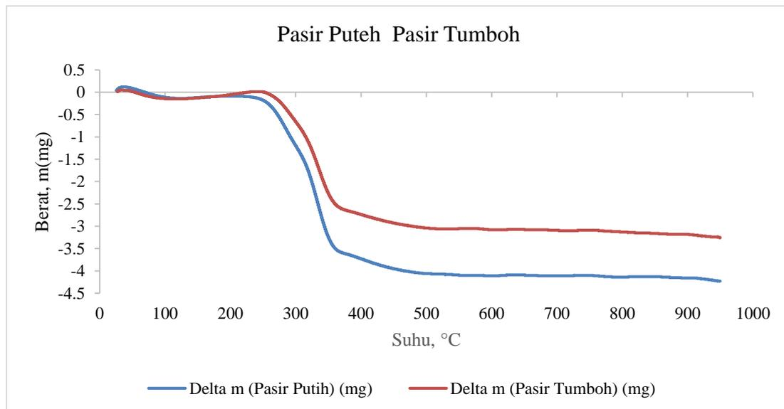
**Figure 3: Weight reduction for both Pasir Puteh vs Pasir Tumbuh rice husks in TGA analysis**
