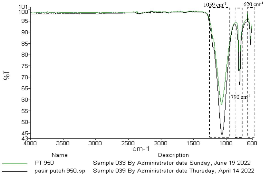
Figure 6: FTIR spectra of Pasir Puteh and Pasit Tumboh crystalline silica
