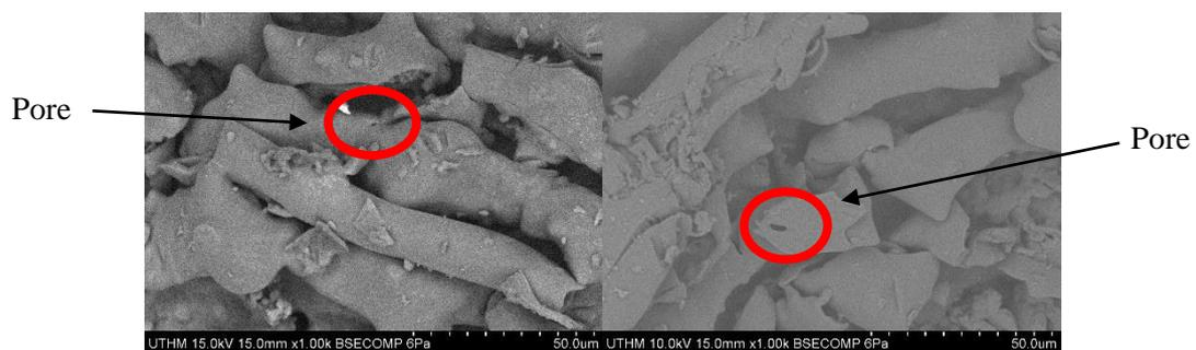
**Figure 2: Morphology of a) Pasir Puteh and b) Pasir Tumboh magnification of x1000 of 950°C sample compare due to the size of the pore (circle).**
