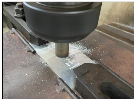
Figure 4 During FSW Process
