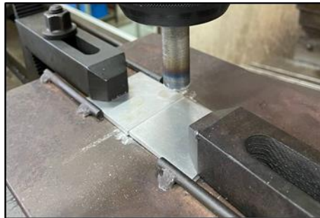
Figure 3 : Specimens are Clamped onto The Jig
