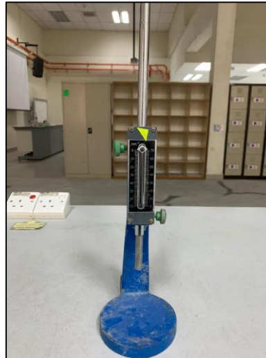
Figure 2: Vicat apparatus experiment for setting time
