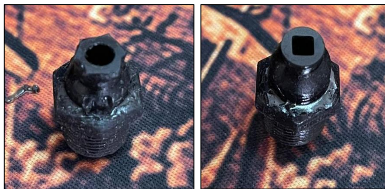
Figure 12: Circular and rectangular shape nozzle
