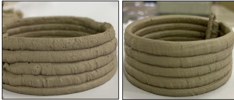
Figure 11: Printed model using 5mm (circular and rectangular nozzles)
