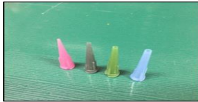
Figure 6: Standard nozzle for clay printing
