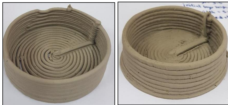
Figure 9: Printed model using 3mm (circular and rectangular nozzles)
