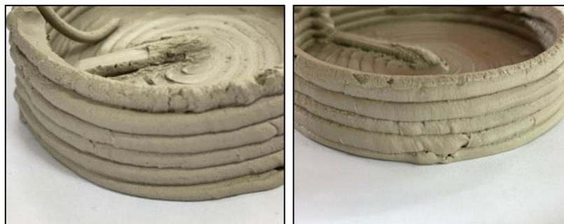
Figure 10: Printed model using 4mm (circular and rectangular nozzles)
