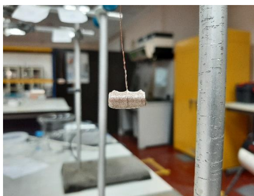
Figure 6: Dipping and hanging of cylindrical samples with copper conductive paint
