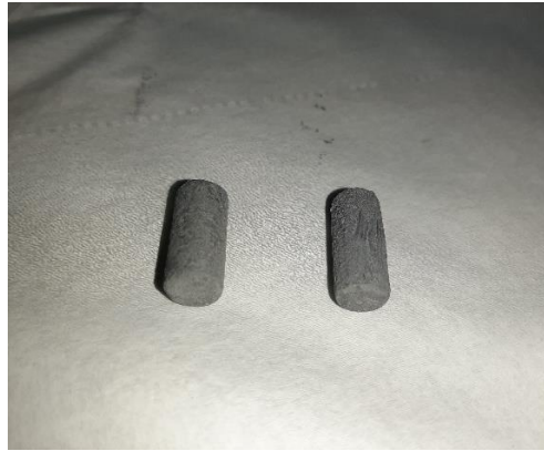
Figure 6: Incomplete and uneven aluminium mixture coating on the samples
