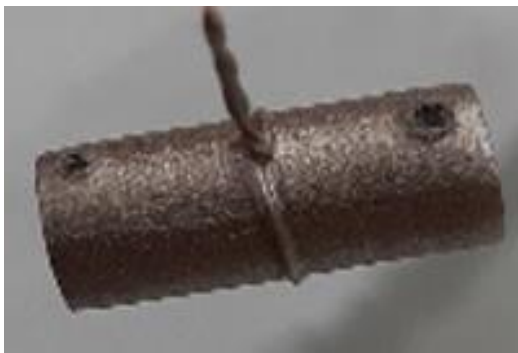
Figure 8: Formation of air bubbles after dipping the paint
