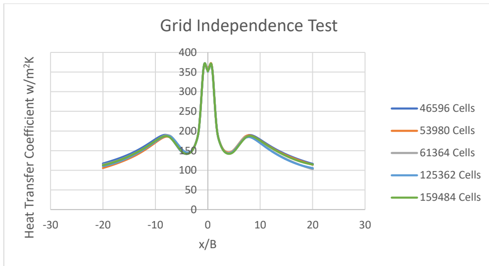
Figure 6: Grid independence test
