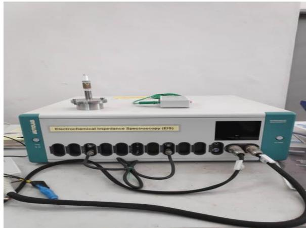
Figure 3: Equipment use for Area Specific Resistance (ASR)
