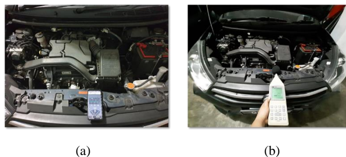
Figure 2: Sound Monitoring on Car Engine Bay using: (a) Smartphone (b) Sound Analyzer (TES-1358)
