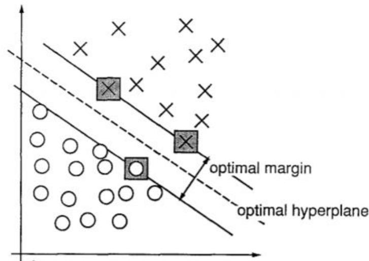
**Figure 7: An example of a separate problem in a 2D space using a SVM. The grey squares defines as a support vector [30]**
