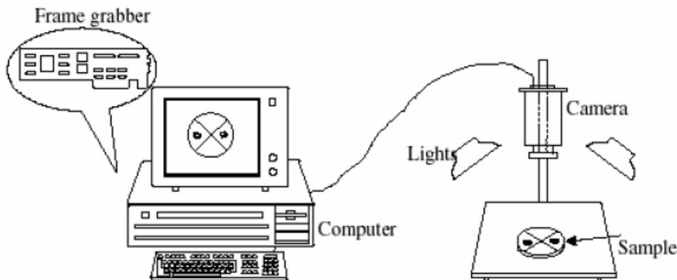
**Figure 1: The component of a computer vision system [10]**
