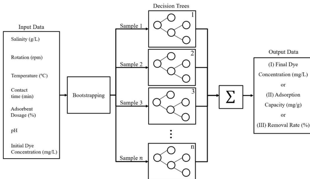
**Figure 8: The schematic diagram of the three models developed using RF prediction [37]**
