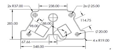
Figure 2: Detail dimension of three dimensional of model
