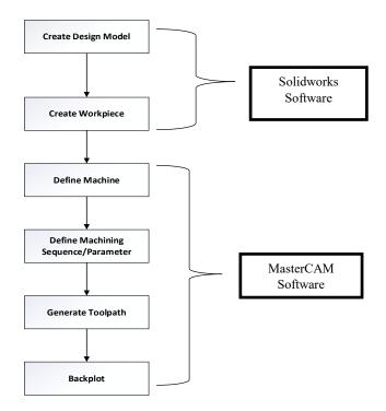
Figure 3: Overall process using MasterCAM software
