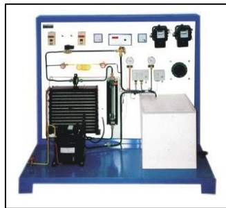
Figure 1.1 : Vapour Compression Refrigeration Test Rig [3]
