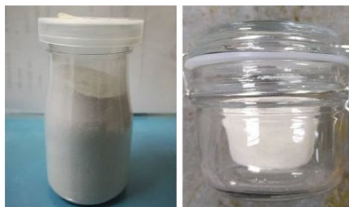
Figure 2: Natural catalyst (left) and calcined catalyst (right)
