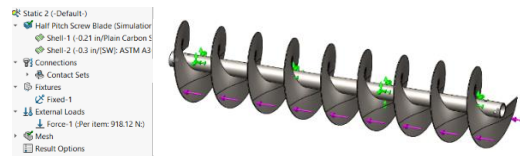
Figure 13: Fixed Geometry and External Load applied on Screw Blade
