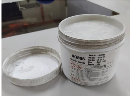
Figure 2: Silver conductive ink (Model: AG 806)
