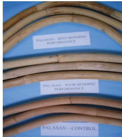
Figure 4: Pictures of bent palasan poles showing bleached poles that did not fail (topmost), those that did fail (middle), and an unbleached control (bottom) (Devera et al., 2009)
