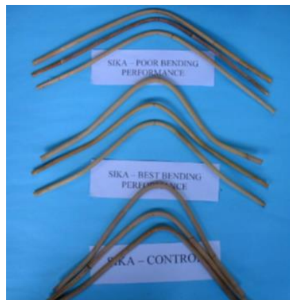
Figure 3: Images of bent bleached sika poles showing samples that readily failed (topmost), samples that did not fail (middle), and unbleached controls (bottom) (Devera et al., 2009)
