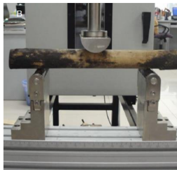
Figure 3: Image of rattan undergoing bending test by Shang et al. (2016)
