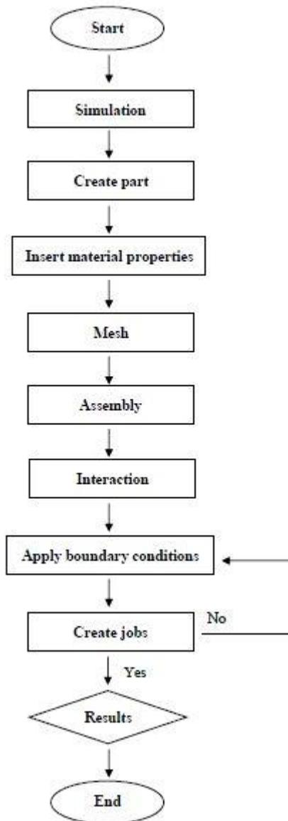
Figure 1 : Flow chart for Simulation using ABAQUS CAE
