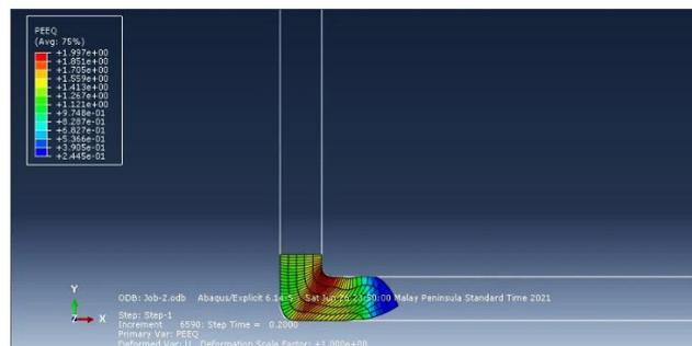
Figure 4 : Analysis for strain distribution at angle 90°
