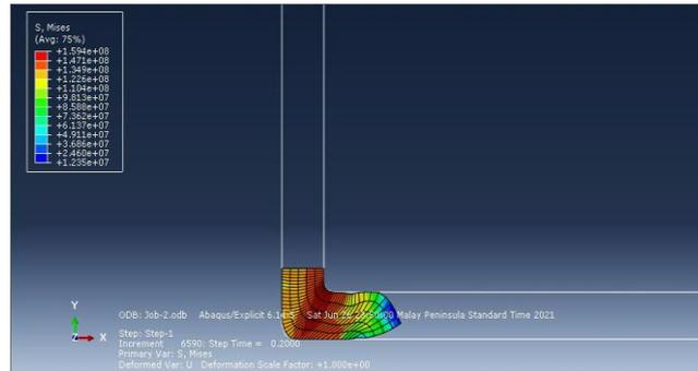
Figure 2 : Analysis for stress distribution at angle 90°
