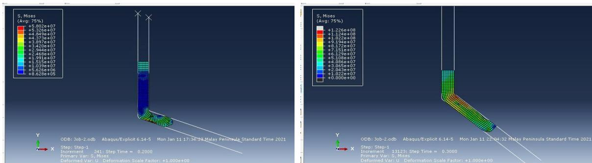
Figure 3 : Analysis for stress distribution at angle 110° and 130°
