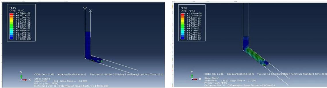
Figure 5 : Analysis for strain distribution at angle 110° and 130°
