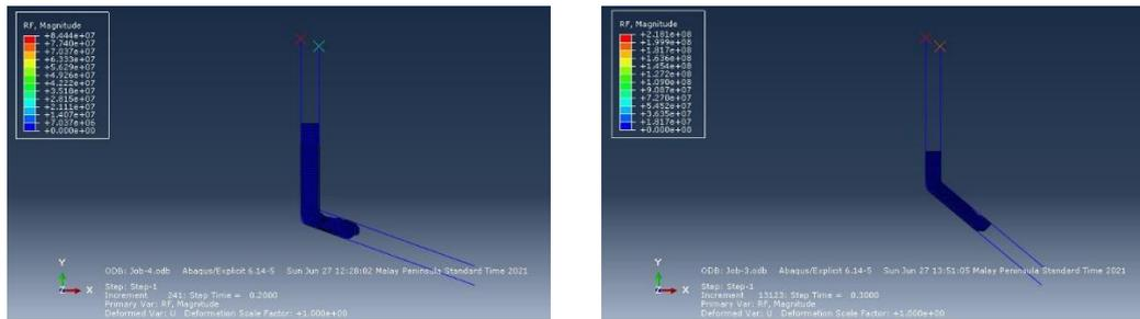
Figure 9 : Reaction force at angle 110° and 130°
