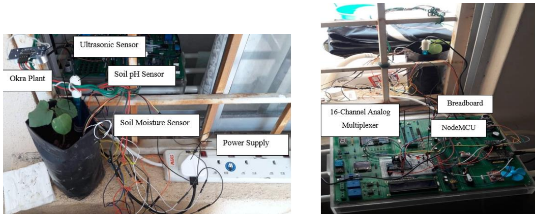
Figure 6: (a) Experimental Setup at the Okra Plant, (b) Experimental Setup at the Micro-Controller
