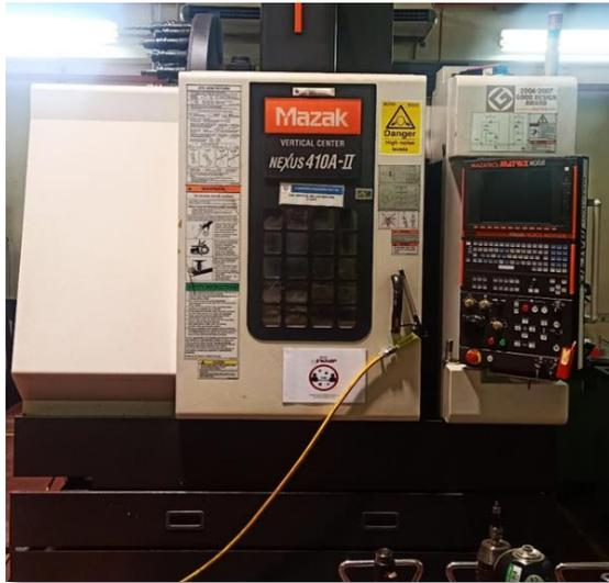
Figure 1: CNC Milling machine
