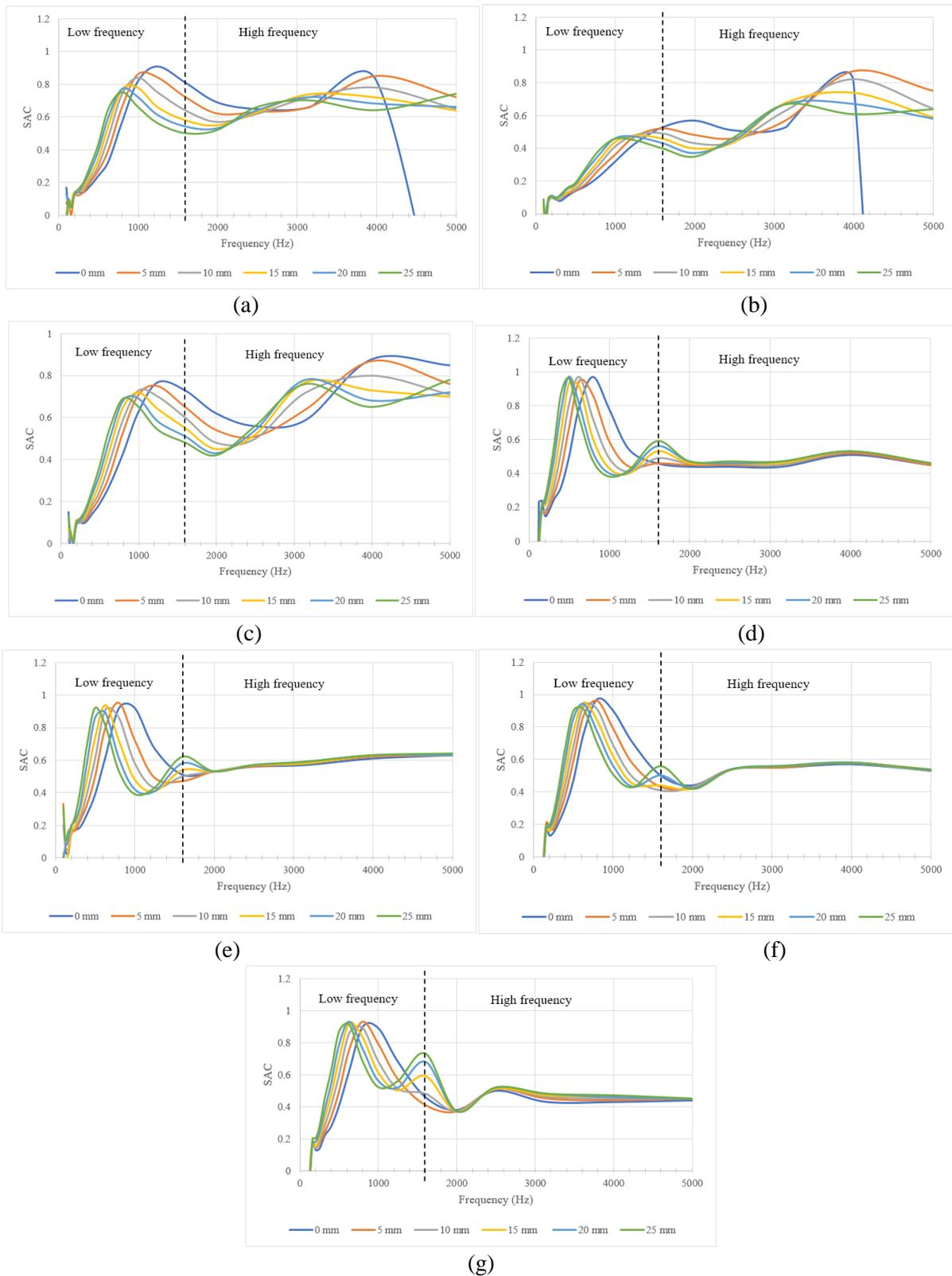
**Figure 6: Influence of air gap in samples made up of smaller stalks**
