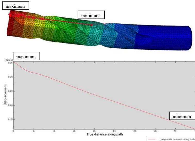
**Figure 6: The path of the cutting tool and graph of Displacement vs. True distance along the path**
