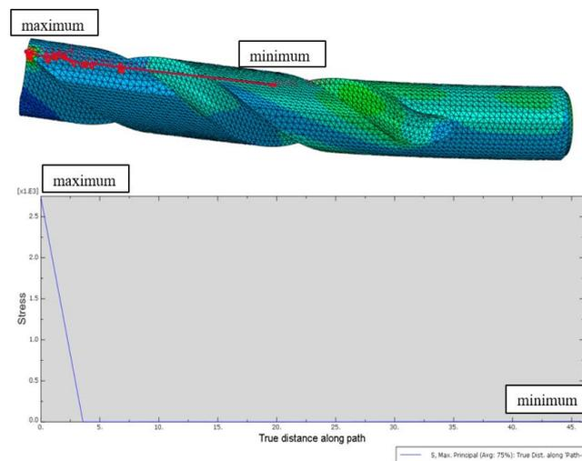
**Figure 5: The path of the cutting tool and graph of Stress vs. True distance along the path**
