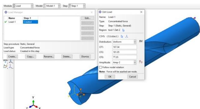
Figure 3: Create a load of cutting tool
