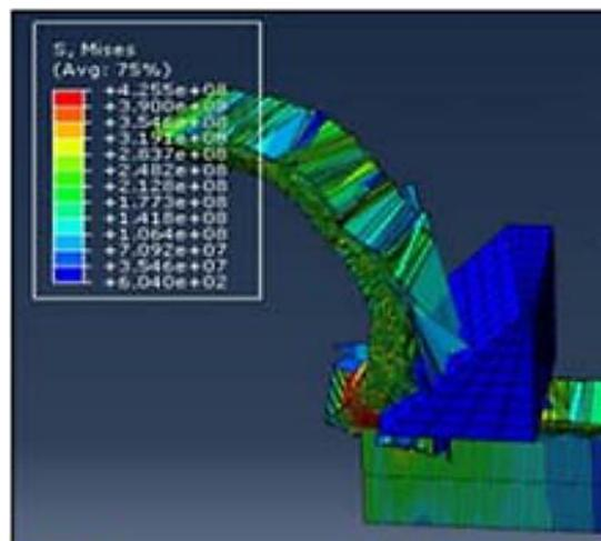
**Figure 7: Chip formation formed in the simulation[7]**
