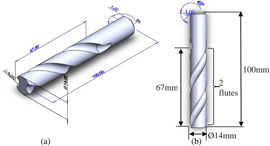
**Figure 2: Two flutes cutter (a) in 3 dimensional (b) in 2 dimensional**
