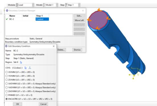
Figure 4: Boundary condition of cutting tool
