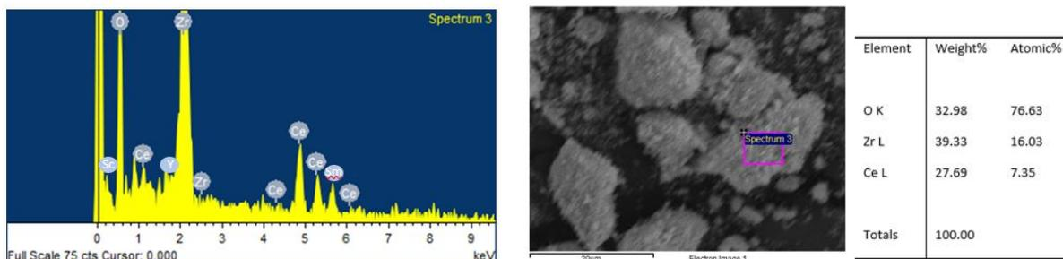
**Figure 6 EDS distribution for calcined YSZ-SDC 70:30 wt%**
