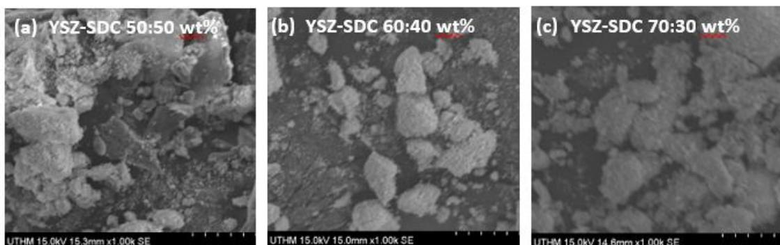
**Figure 1 SEM morphologies of calcined (a) YSZ-SDC 50:50 wt%, (b) YSZ-SDC 60:40 wt% and YSZ-SDC 70:30 wt% at temperature 950°C**
