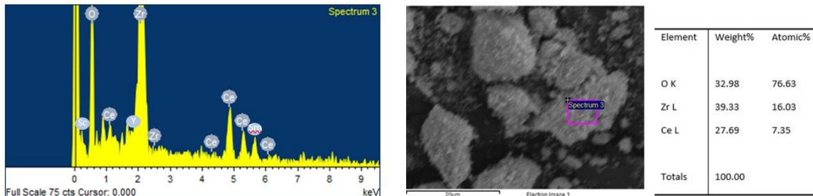
**Figure 5 EDS distribution for calcined YSZ-SDC 60:40 wt%**
