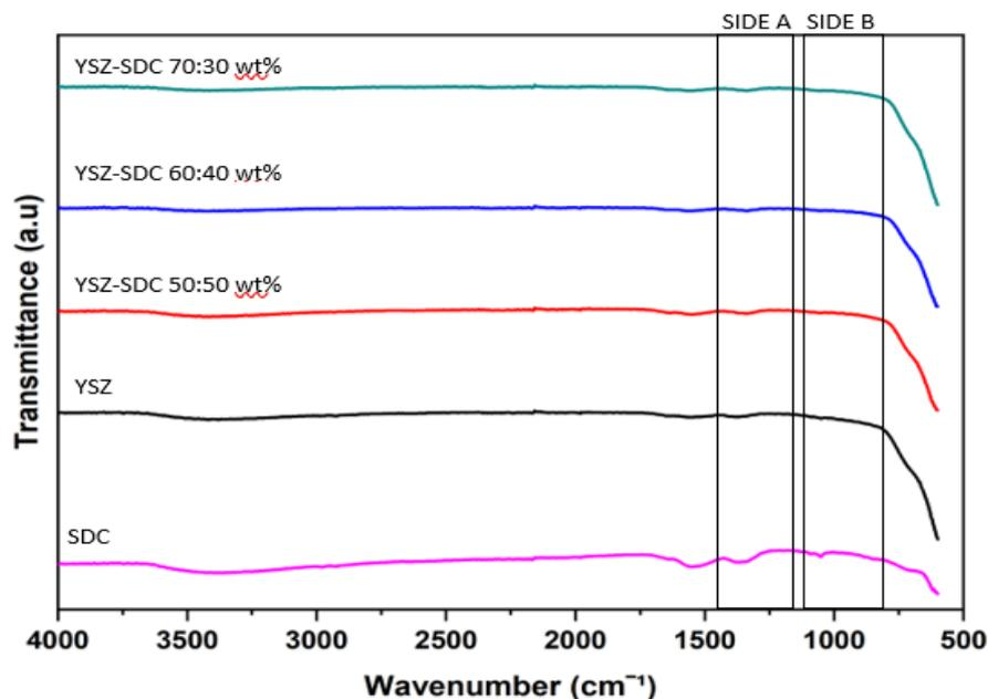
Figure 3 FTIR pattern of calcined SDC, YSZ and YSZ-SDC powder
