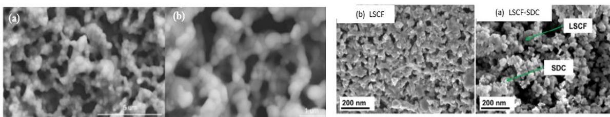
**Figure 8 SEM images for calcined LSCF-SDC with 50:50 wt% (a) and (b) view powder with different magnification at 1150°C [11].**
