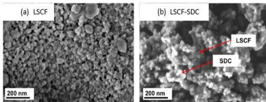
**Figure 7 FESEM images of calcined (a) LSCF and (b) LSCF-SDC of 50:50 wt% powder at 700°C [10]**
