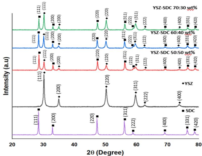
Figure 2 XRD pattern of calcined SDC, YSZ and YSZ-SDC powder with composition 50:50, 60:40 and 70:30 wt%
