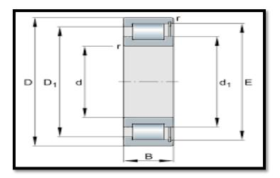
Figure 2: Cross section for the bearing [8]
