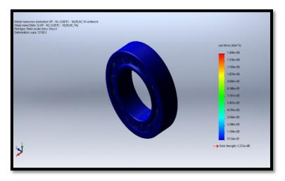
Figure 3: Equivalent force on the cylindrical roller bearing without lubrication by SOLIDWORKS
