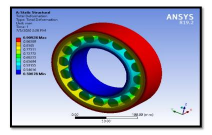
Figure 7: Total deformation on the cylinderical roller bearing using oil lubrication
