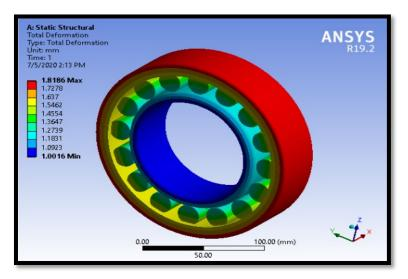
Figure 6: Total deformation on the cylinderical roller bearing using grease lubrication
