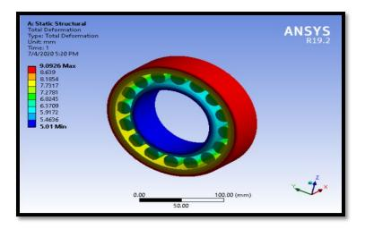
Figure 5: The total deformation on the cylinderical roller bearing without lubrication by ANSYS
