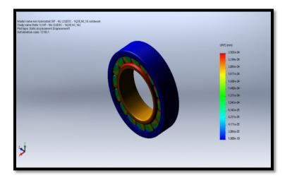
Figure 4: Total deformation on the cylindrical roller bearing without lubrication by SOLIDWORKS
