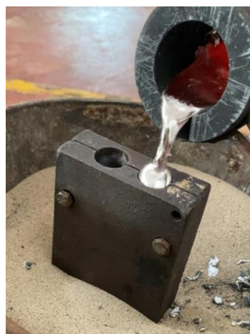
Fig. 3 Pouring molten Al-Cu alloy into cylindrical steel mould.
