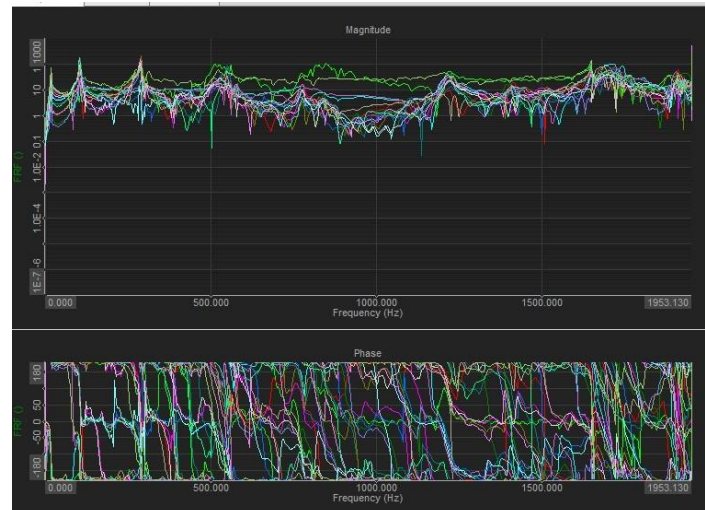
Fig. 1 Frequency Response Function (FRF) Graph for mild steel beam.
