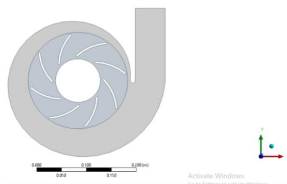
Figure 4: Design Modeler of 8 blades at 40^\circ angle
