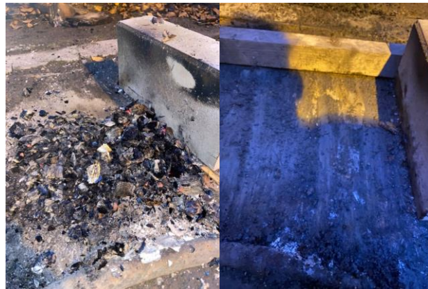
Fig 13: Before and After Use Prototype Multi-Sprayer Ash Vacuum Cleaner
