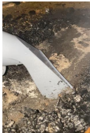
Fig 12 : Testing Suction Vacuum on Ash Burn Particle
