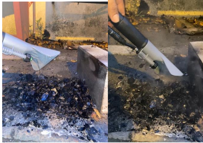
Fig 11: Testing Multi-Sprayer Nozzle On Ash Burn
