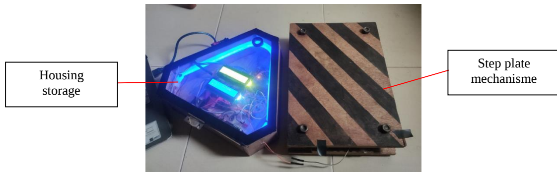
Fig. 5 Fully assembled prototype with simple mechanism
