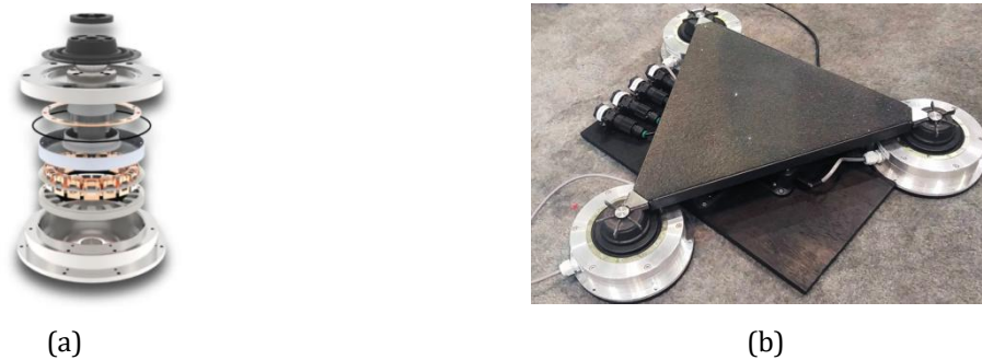
Fig. 3 a) Exploded view of electromagnetic hybrid system, b) Full assembled of electromagnetic hybrid system
