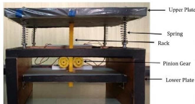
Fig. 1 Mechanism of rack and pinion gear
