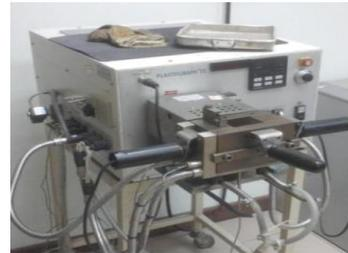
**Figure 2: Rotary Plastograph Brabender Mixer**
