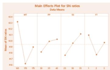
**Figure 4: Main Effect Multiple S/NQP ratio for 0wt.% GS**
