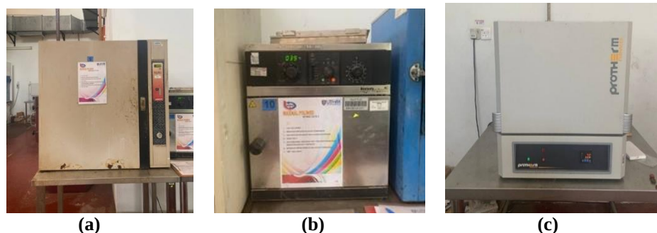
Fig. 5 Equipment used to expose specimens to temperature (a) Drying oven; (b) High capacity oven; (c) Furnace
