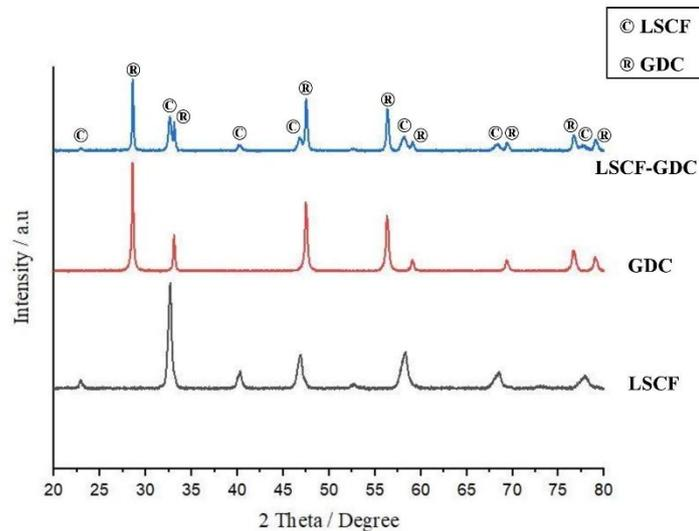
**Figure 2: XRD Pattern of Composite Powder Cathode LSCF-GDC**
