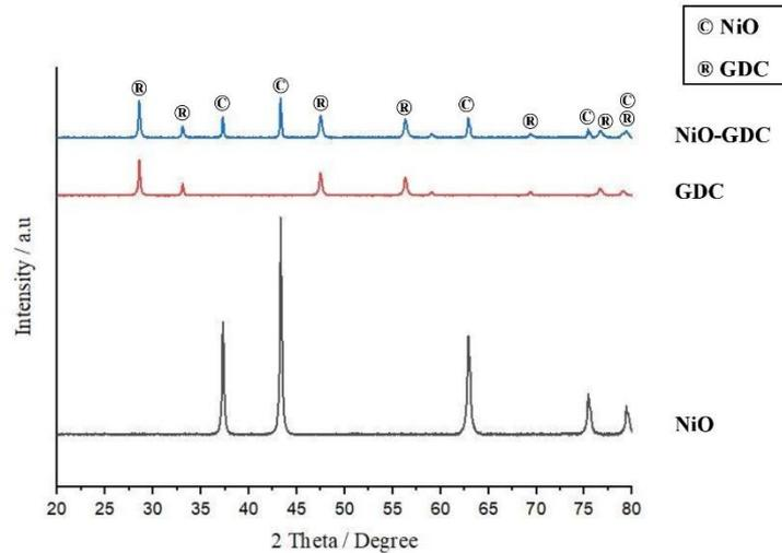
**Figure 1: XRD Pattern of Composite Powder Anode NiO-GDC**
