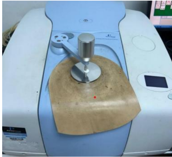
Fig. 2 Fourier Transform Infrared Spectroscopy (FTIR)
