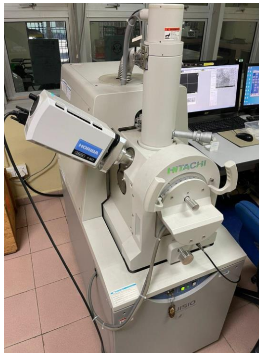
Fig. 3 Scanning Electron Microscope with Electron Dispersive Spectroscopy (SEM-EDS)
