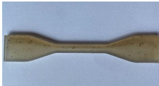
Fig 4 A Dog Bone Bar Specimen
