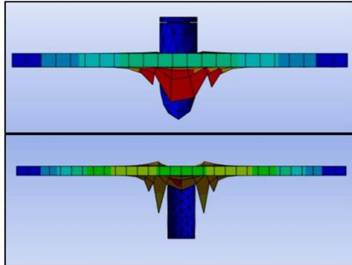
**Figure 7: Failure mode of geometry by hemispherical bullet and blunt bullet with velocity 1500m/s**
