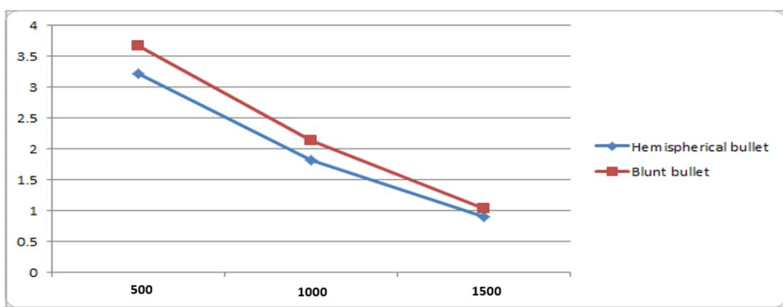
**Figure 5: Graph of time taken for bullet to complete penetration at a different velocity**
