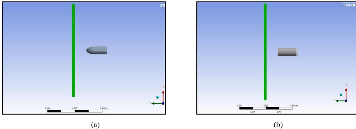
**Figure 1: Finite element model of projectile and AHSS target plate (a) Hemispherical nose shape (b) Blunt nose shape**
