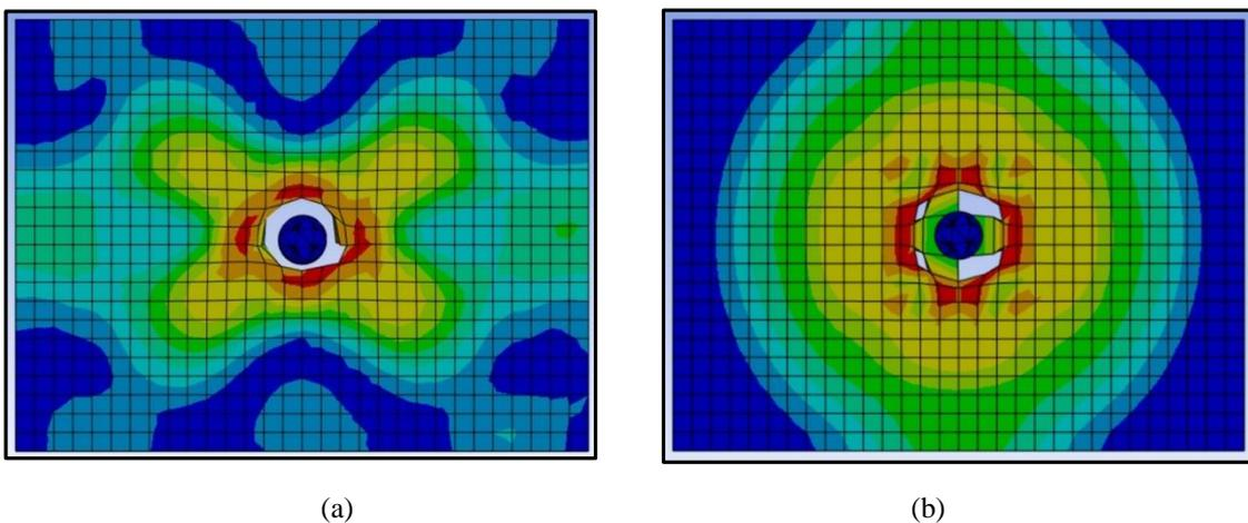
**Figure 6: Top view images of post penetration of projectile (a) Hemispherical nose shape (b) Blunt nose shape**
