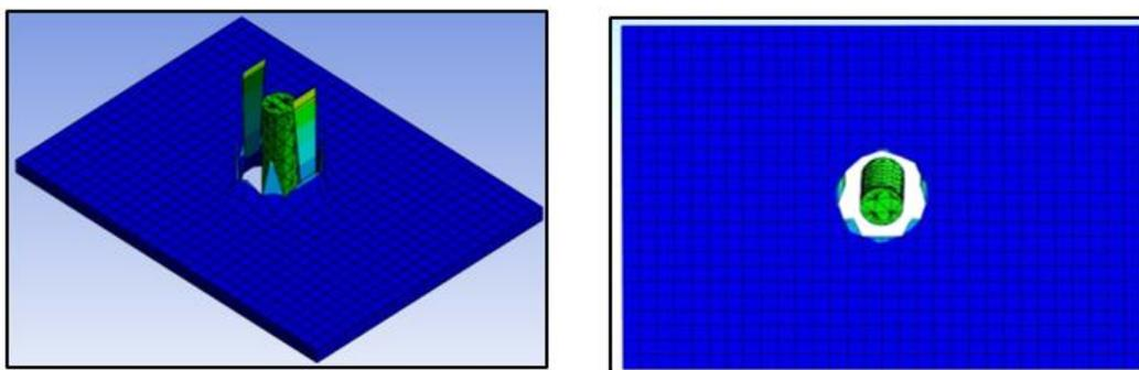
**Figure 4: Failure mode of model impacted by blunt bullet at a velocity of 1000m/s**
