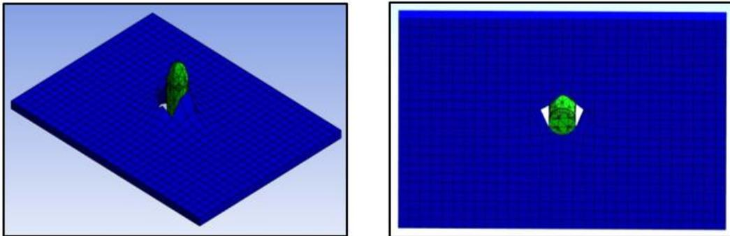
**Figure 3: Failure mode of model impacted by hemispherical bullet at a velocity of 1000m/s**
