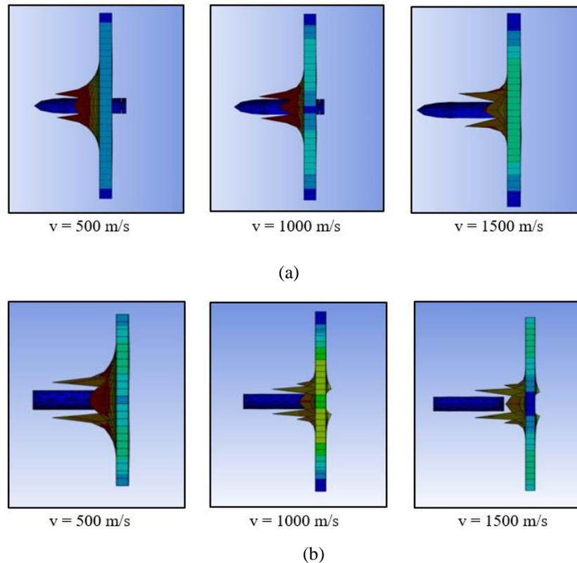
**Figure 2: Penetration of projectile at different velocity impact (a) Hemispherical projectile impact
