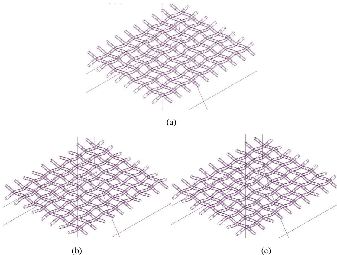
**Figure 2: Model for Woven Wire Mesh Screen (a) Plain Weave (b) Twill Weave (c) Satin Weave**
