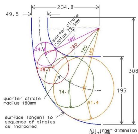
**Figure 1: Construction Line of Curved Diffuser [10]**
