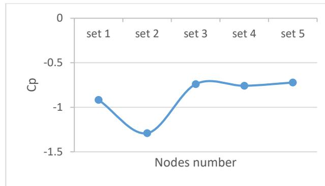
**Figure 3: Grid Independence Test (GIT) for Realizable Model**
