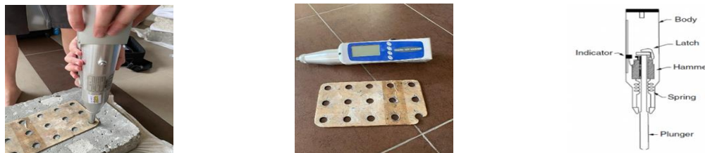
Figure 4: Rebound Hammer Test for Specimens
