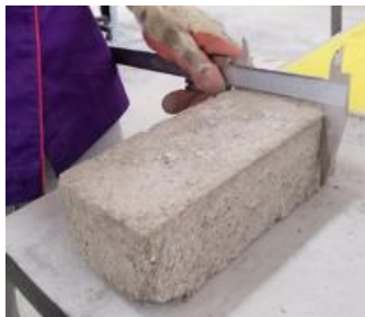
Figure 11: Brick is measured using vernier calliper
