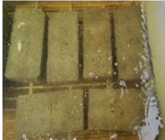
Figure 10: Bricks are immersed into water tank
