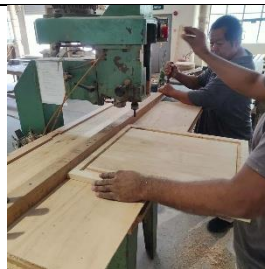
Fig. 11 Thinned panel to create internal cavities
