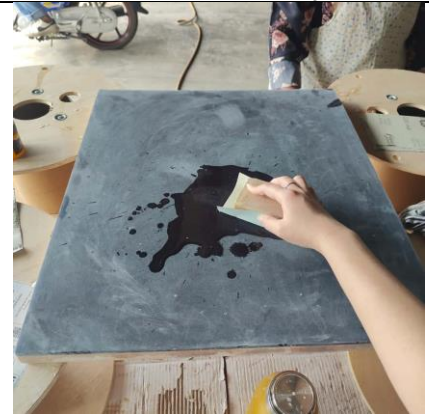
Fig. 24 Process Sanding Epoxy Resin Surface
