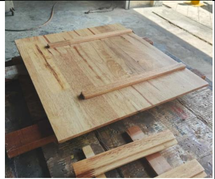
Fig. 33 Process Applying Second Layer of Matt Topcoat
