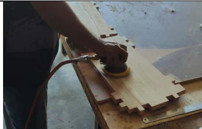
Fig. 26 Process Sanding with 240-Grit
