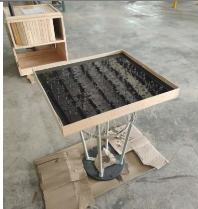
Fig. 23 Process Curing Epoxy Resin
