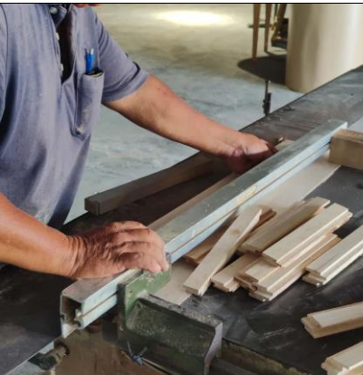
Fig. 13 Tambour Door Tongue and Groove Joint Cutting
