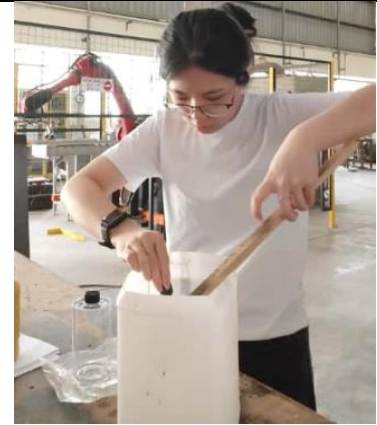
Fig. 21 Process Mixing Epoxy Resin with Black Colour Dye
