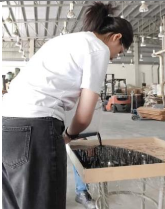
Fig. 22 Process Pouring Epoxy Resin to Tabletop
