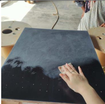
Fig. 25 Process Applying Natural Beeswax on Epoxy Resin Surface
