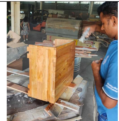
Fig. 30 Process Applying Second Layer Coat of NC Sealer
