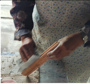
Fig. 31 Process Lightly Sanding for Matt Topcoat
