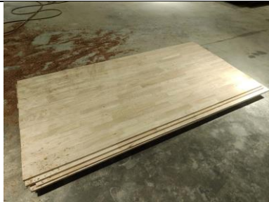
Fig. 7 Main Required Material (Rubberwood panel sized 8ft*20mm*4ft)
