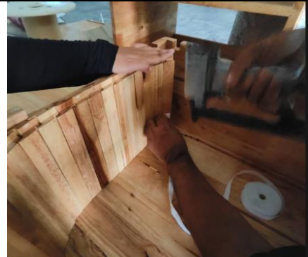
Fig. 36 Process Connected Tambour Door Slats using Polyester Webbing
