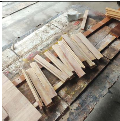
Fig. 29 Process Lightly Sanding with 320-grit Sandpaper
