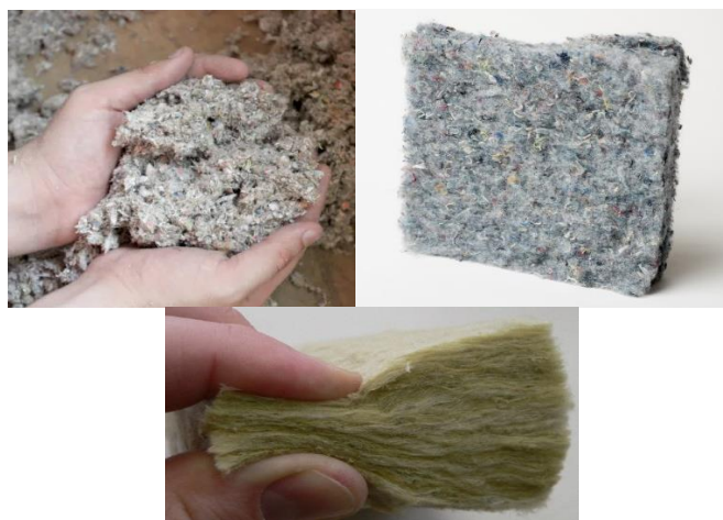
Figure 3 (a) (b) (c): Formaldehyde-free insulation: Cellulose insulation, cotton insulation and wool insulation
