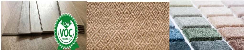
Figure 1 (a) (b) (c): Example of low-emitting flooring: Vinyl flooring, Sisal Carpet and Nylon Carpet
