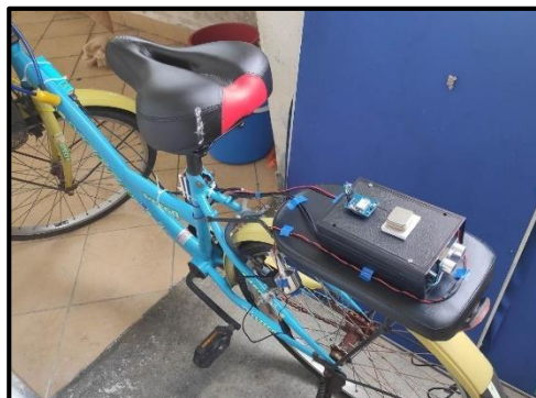
Figure 7: Connection of dynamo.
