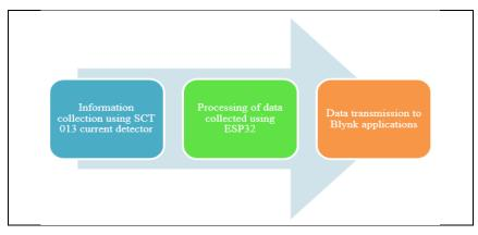
Figure 1: Block diagram of energy consumption monitoring system using IoT
