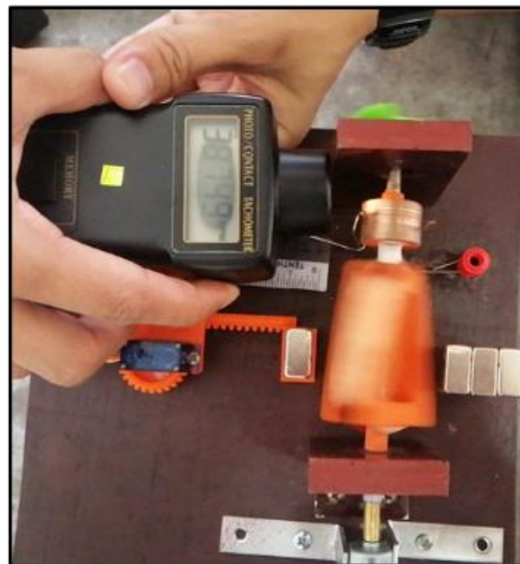
Figure 12: The speed of the motor proved by the tachometer result when the air gap effect by the magnet position
