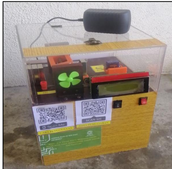
Figure 9: The model direct current motor based on Fleming Left Hand Rule
