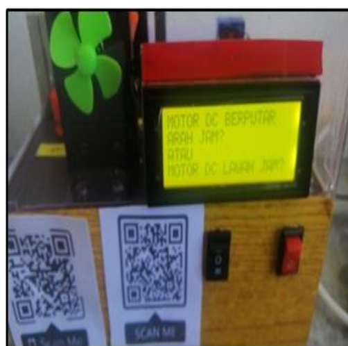
Figure 10: The Fleming Left Hand Rule was proved by the experiment follows by the instruction of the LCD2004
