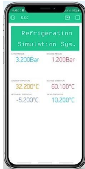
Figure 3: Blynk Application equipped with Internet of Things
