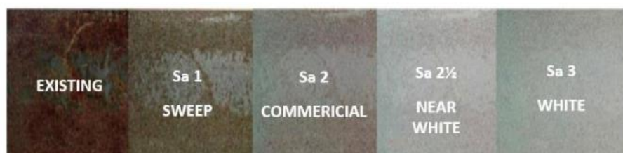
Figure 1: Standard Profile Surface Preparation
