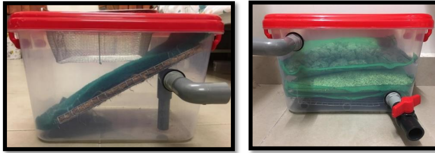
Figure 2: Prototype design of a water filtration system and recycling system for flushing toilet
