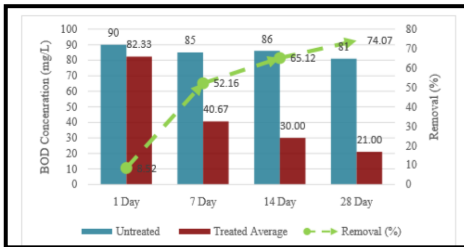
Figure 9: Graph comparison of testing biochemical oxygen demand
