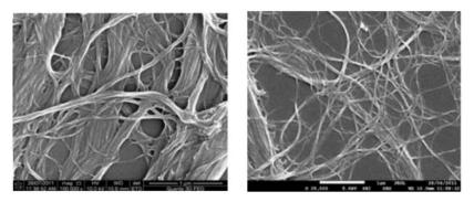
Figure 3: SEM images of MFC (left) and NFC (right) [25]
