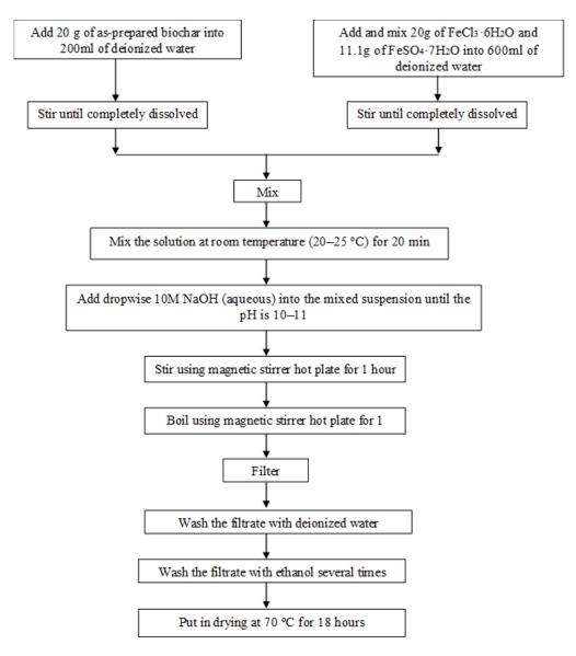
Figure 5: Flowchart preparation of magnetic biochar
