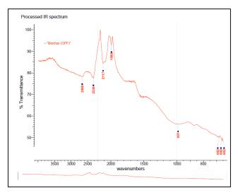
Figure 6: FTIR Spectra of Biochar
