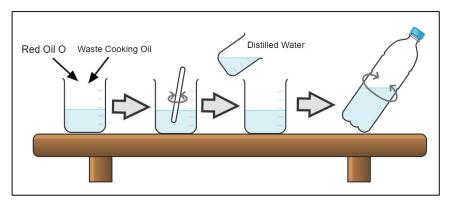
Figure 1: Procedure for preparation of synthetic waste cooking oil
