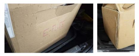
Figure 15: Defects on E-Flute PCTB at 60 km/hours
