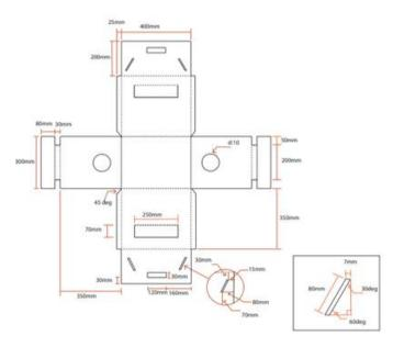
Figure 11: Die cut drawing of PCTB
