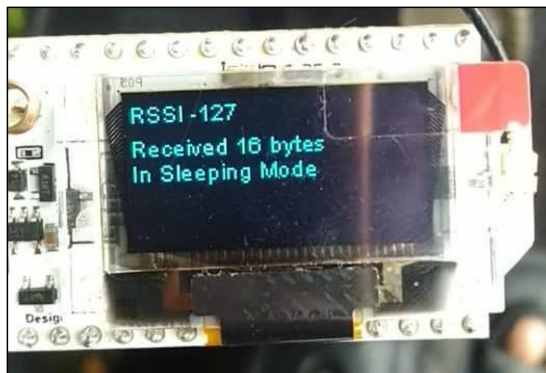
Figure 11: Receiver Node's OLED panel display (Sleep mode)
