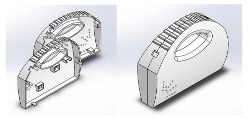
Figure 7: Modified design of hand mixer
