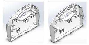
The original design used four screws as the fastener for the rear casing and front casing. Meanwhile, the modified design used the snap-fit concepts where can be differentiated between the pictures above. A few parts can be reduced through the rear and front casing redesign, such as the four screws. Snapfit used was not added to the raw material used for the product as it replaced the removed slot for the screw at both rear and front casing.
