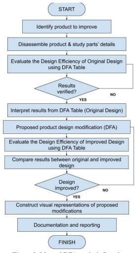
Figure 3: Manual DFA analysis flowchart
